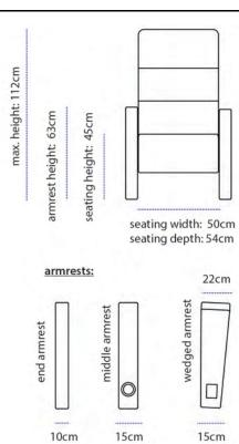
dimensions may vary due to leather, foam thickness and density, covering materials and position of reclining mechanism. Allow for small deviations - especially for row configurations
